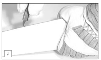
Regularly inspect the bearing surfaces of the guide bar for damage, and clean them with a suitable tool.
